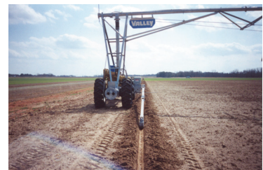
Furrow Guidance shoe will assist in the maintenance of the furrow as shown, but if the furrow is damaged it must be repaired.
