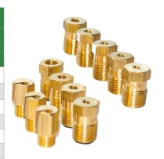
The wide range of brass or plastic nozzles offer a number of possible combinations. This sprinkler is designed to work under a flow range between 3 and 14 gpm, at pressures between 25 and 65 PSI and a cover range between 42 and 60 feet of diameter. The VYR-35 can work with one or two nozzles, both nozzles are 26 degree angle to the horizontal plane. Their average time of rotation comes to be approximately 40 sec.
