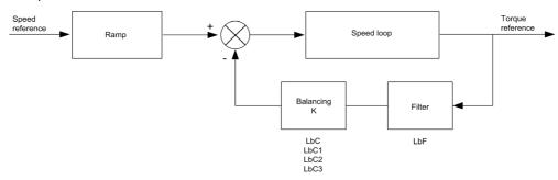
The load sharing factor K is determined by the torque and speed, with two factors K1 and K2 (K = K1 x K2).
