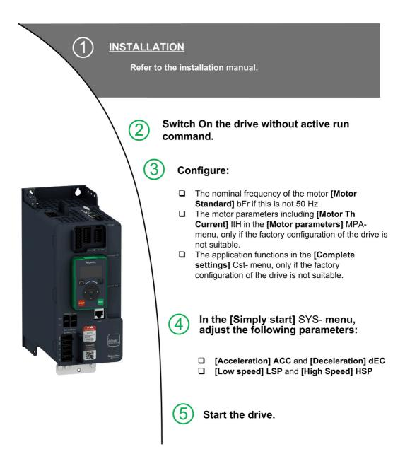
Drive systems may perform unexpected movements because of incorrect wiring, incorrect settings, incorrect data or other errors.
