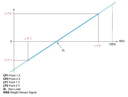
This curve can represent a weight sensor where zero load on the motor occurs if the load is not zero.
