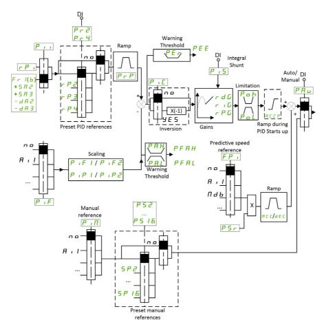
The PID feedback needs to be assigned to one of the analog inputs Al1 to Al5 or a pulse input, according to whether any I/O extension module has been inserted.
