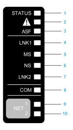
Following table provides the details of the drive status LEDs:
