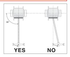
**C.** After having oriented the reel, secure it by the pin into one of the special stop dogs; to obtain the correct machine inclination use it in one of the reel drive gear positions.
