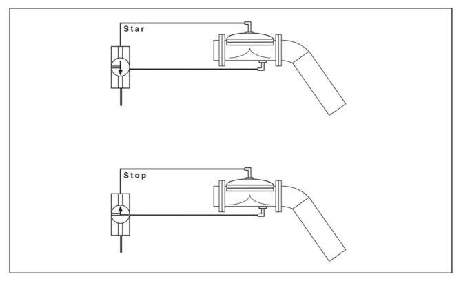
On the water piloted shut off valve kit produced after 1/9/96 a ball valve with big diameter has been installed before the piloted valve. This is used to drain the water from the reeled in hose when it is unreeled by the tractor. To drain the hose in this way, open the ball cock before unreeling the hose and close it when the hose has been unreeled.
