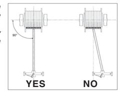
**C.** After having oriented the reel, secure it by the pin into one of the special stop dogs; to obtain the correct machine inclination use it in one of the reel drive gear positions.
