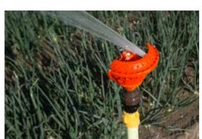
The PC-R2000WF is a Part-Circle Rotator that distributes water in a 180 degree arc. It is intended to irrigate the edge of a field where full circle Rotators are used in the interior.
