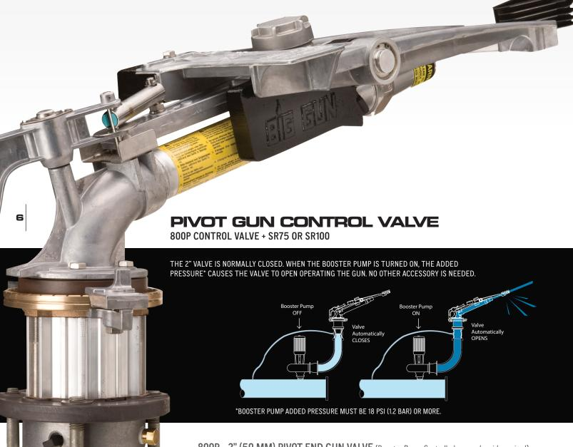
**800P - 2" (50 MM) PIVOT END GUN VALVE** (Booster Pump Controlled - no solenoid required) Medium Pressure sleeve (18-80 psi) includes ball drain/vent, 2 rubber drains, and 1/4" tube fitting in jacket
