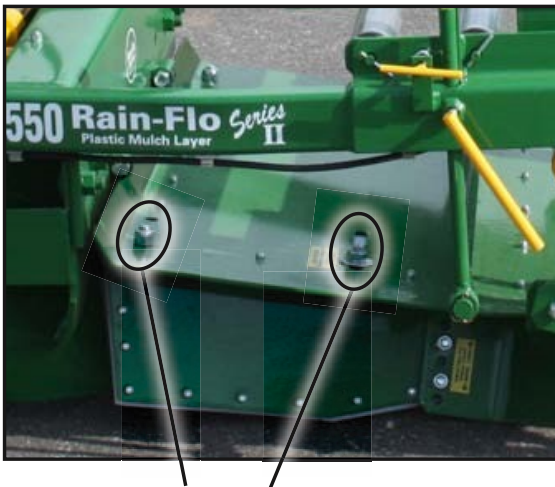
(No.3) Remove bolts from bed press side plates and move to appropriate setting. NOTE; For straight beds, each side must be equally adjusted.
