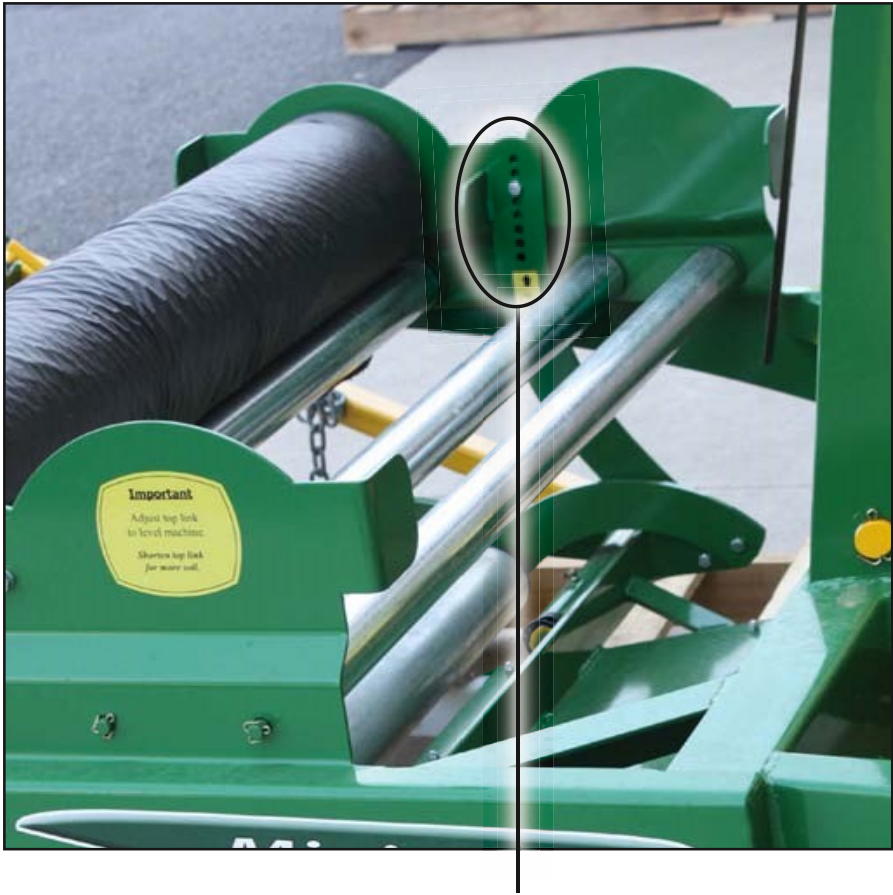
Bed Height Adjustment (Move up for higher bed; down for lower.)
