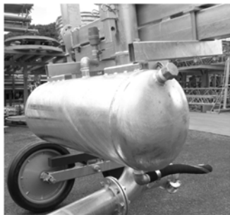
Ballast water tank
