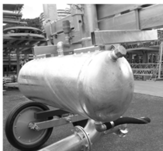
Ballast water tank
