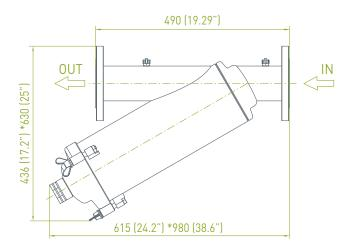
**Dim: mm (inch)** \*Approx. length required for maintenance
