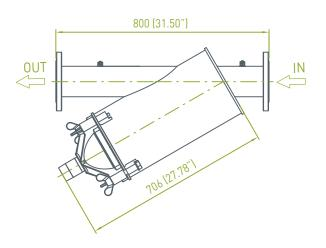
**Dim: mm (inch)** \*Approx. length required for maintenance 4" Compact In-Line **Typical Installation Drawing**
