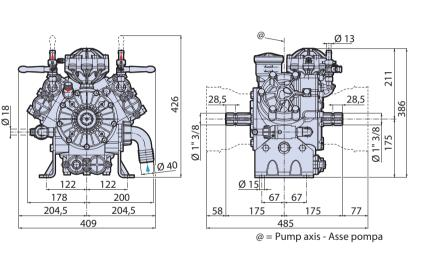
In C/SP pumps the value  $\Delta$  17 is reduced to 15 with the seal ring flange mounted on the pump body. N.B. Remove the seal ring flange code 1400140 before fitting the reduction gear to the pump.
